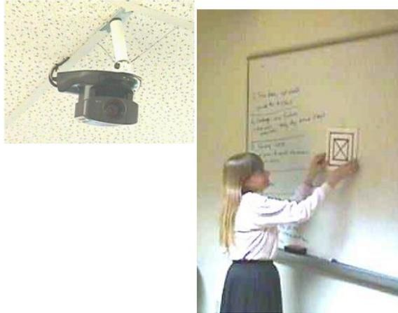
**Figure 1. The PARC ZombieBoard whiteboard scanner. The pan/tilt/zoom video camera is mounted in the ceiling. The user is placing a magnetic pre-drawn “scan whiteboard” command button.**
